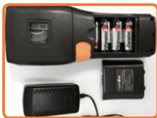
Supplied with 9V power supply (also runs off 6 AA batteries)
